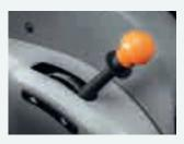
The ergonomically positioned creeper engagement lever falls naturally to hand (Creeper option only).
