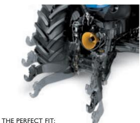
New Holland's T6000 range is designed to incorporate a fully integrated, factory fitted, front linkage and PTO. All linkage and PTO controls are positioned inside the cab for ease of operation. Purpose developed for T6000 tractors, the linkage will lift up to 3090kg. Linkage arms can be folded when not in use, or can be used to carry the new mono block front weight pack.
