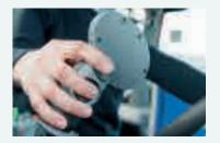
The button on the rear of the CommandGrip  $\ensuremath{^{\text{TM}}}$  gives access to further functions.
