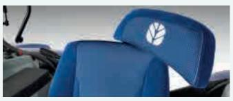
Both the Dynamic Comfort and Comfort seats benefit from innovative swiveling backrest, designed to provide upper back support and significantly increases comfort when the seat is turned to monitor rear mounted implements.
