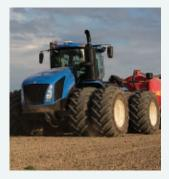
Grain cart applications with VF dual tyres (Row Crop Frame shown) allow for high-speed, low-pressure inflation, which lessens soil compaction while boosting fuel economy. Through less compaction, the T9 Series tractor improves your harvest and yields the following year.
