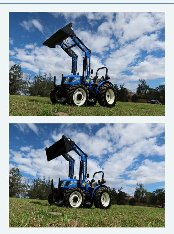
A New Holland APs30 Front End Loader system has been developed as a local, Dealer installed option. This takes advantage of the TT3.50's useful hydraulic output as well as the generous wheelbase and rated axle capacities.
