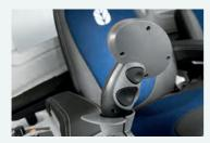
Shift button and ground speed unlock (behind).
