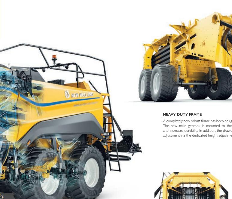
A completely new robust frame has been designed to manage the higher density loads this baler experiences. The new main gearbox is mounted to the top beam which reduces crop accumulation underneath and increases durability. In addition, the drawbar is not part of the main frame, in order to facilitate height adjustment via the dedicated height adjustment rods, perfect when working with different tractors.
