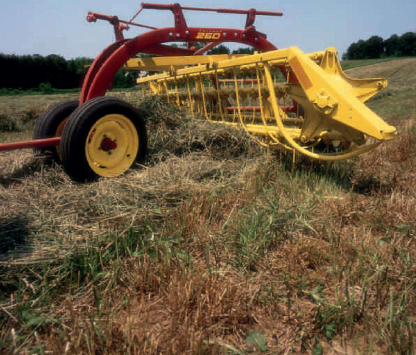
New Holland Rolabar® rakes let you feed cleaner hay and more of it. Offset wheels are set close to the basket, so tines follow the ground contour closely to pick up all the hay but leave dirt behind.
