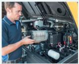
• The engine air filter is easy
