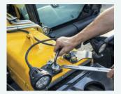
Adjusting the telescopic boom pads has been simplified, a simple nut screw and lock nut system making adjustment quick and easy
