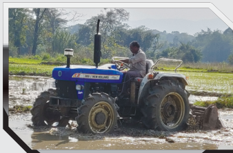
Puddling - Rotavator with 4WD Tractor
