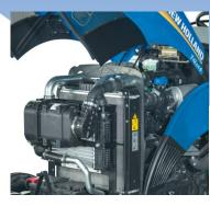
The engine air filter is easy to check, clean or replace, with no need for tools.
