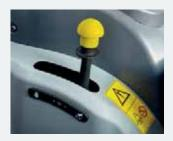
A dedicated Ground Speed PTO can be specified. Perfect when spreading slurry or lifting turf. Protect your implements and tractor with the soft-start PTO setting. Auto PTO will disengage and reengage the PTO during a headland turn.
