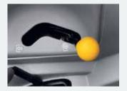
On Synchro Shuttle™ cab models, the PTO is positively engaged courtesy of an ergonomically positioned servo-assisted lever for effortless actuation.
