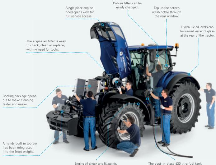
Engine oil check and fill points are easy to reach, with no need to lift the hood. This makes routine checks faster and servicing simpler. The best-in-class 630 litre fuel tank means you can work the whole day long and well into the night without the need to refuel. True 24 hour productivity courtesy of the T7 Heavy Duty range.
