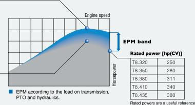
Rated powers are a useful reference but are usually surpassed by the max power figures during work, with or without EPM active.
