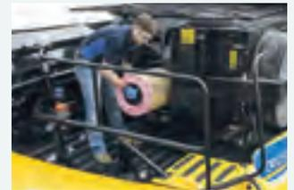
The air filter is easily accessible from the engine platform.
