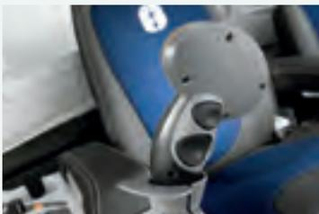
Shift button and ground speed unlock (behind).
