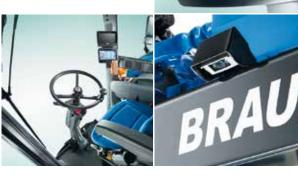
**REMOTE CAMERA READY** The machines are fitted with two cameras and a third can be added to enhance visibility and view machine functions. Images are displayed on a dedicated colour monitor that fits to the top of the IntelliView screen.
