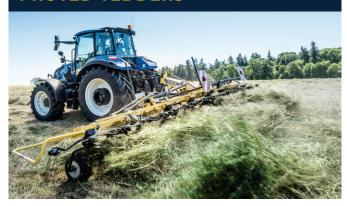
The ProTed™ range of tedders is available in both mounted and trailed specifications. The three mounted models feature working widths of 5.4, 6.9 and 8.8 metres, and for those looking to optimise the horsepower/width ratio, a trailed tedder is also available in the largest 8.8 metre width.
