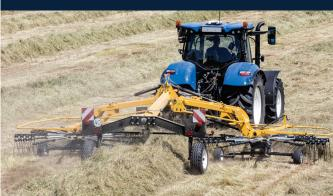
ProRotor™ double rotor rakes ensure central crop delivery. Benefitting from high ground clearance, this range is ideal when working with large swaths of dense crop. Available on the 760 and 820 the cardanic rotor suspension technology means that the rotors can move both laterally and fore-aft freely for efficient operation.
