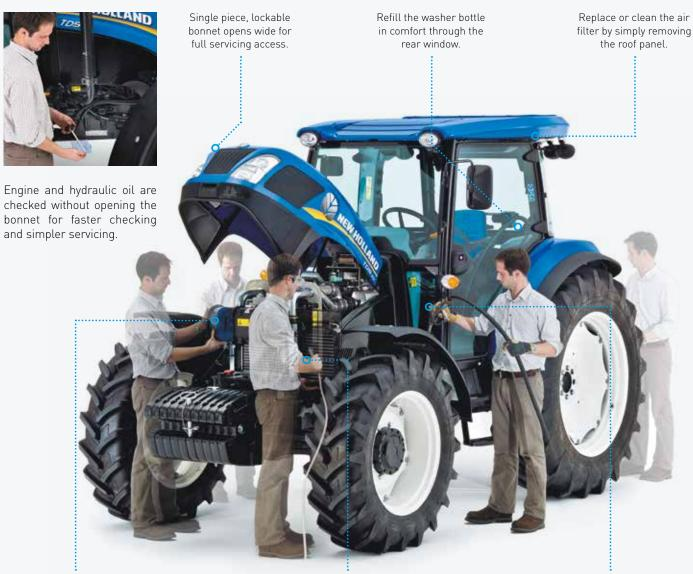
Check, clean or replace the air filter quickly and easily by undoing just four clips.
