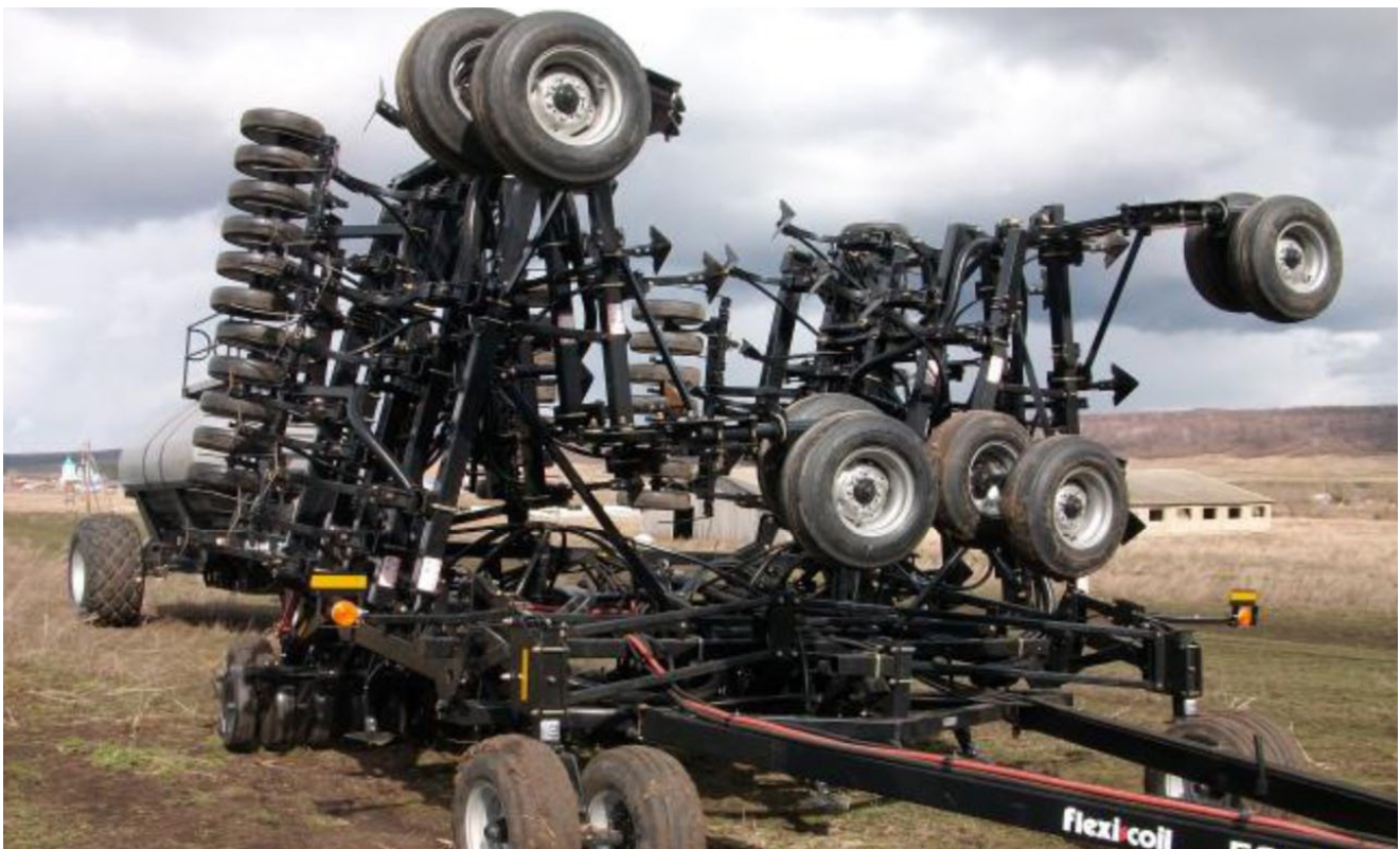
Drill: sweeps are not the right tool in canola. Openers are the better choice.
