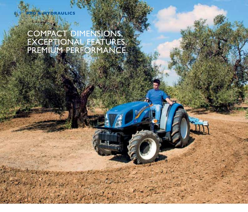
Lighter and shorter than the award winning specialised T4000F/N/V series tractors, the new T3F machines are on a par with their "big brothers" in terms of features. Hydraulic rear hitch with two external hydraulic rams, lift capacity of up to 2277kg and Lift-O-Matic™ system supplied as standard. Two separate pumps for the hydraulic circuit and steering. Up to 3 remote valves. Servo-assisted PTO with up to 3 speeds.
