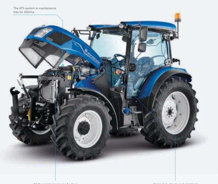
All the maintenance can be done on one side, all is located on the left to facilitate the access
