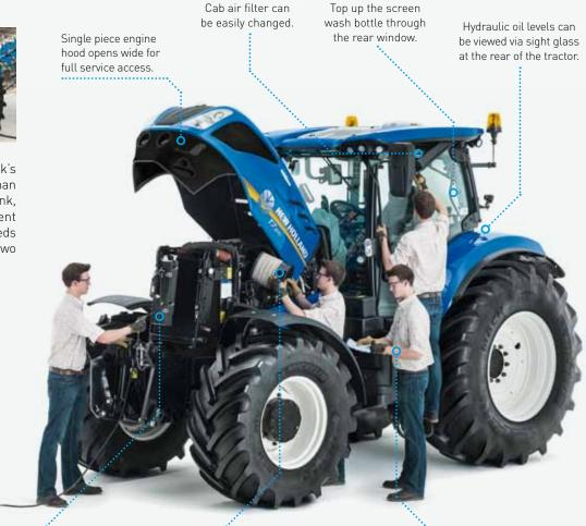
Cooling package opens out to make cleaning faster and easier. The engine air filter is easy to check, clean or replace, with no need for tools. Engine oil check and fill points are easy to reach, with no need to lift the hood. This makes routine checks faster and servicing simpler. You will also still be able to enjoy the long 600 hour service intervals that you've come to expect of New Holland.
