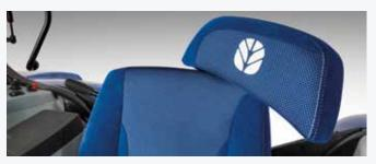
All seats benefit from innovative swiveling backrest, designed to provide upper back support and significantly increases comfort when the seat is turned to monitor rear mounted implements.
