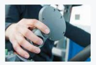
The button on the rear of the CommandGrip  $\ensuremath{^{\text{TM}}}$  gives access to further functions.
