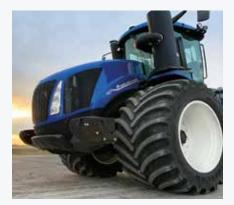
When equipped with LSW1250/35R46 singles, the overall width measures about 150 inches or 12.5 feet. This narrow roading width, in combination with a light footprint, provides a middle ground.
