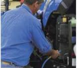
The cooling package slides out for simple and efficient cleaning.
