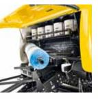
Integrated prop to support a roll of net when changing it from ground level.
