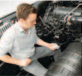
Engine and hydraulic oil can be checked at a glance, without the need to open complicated panels.
