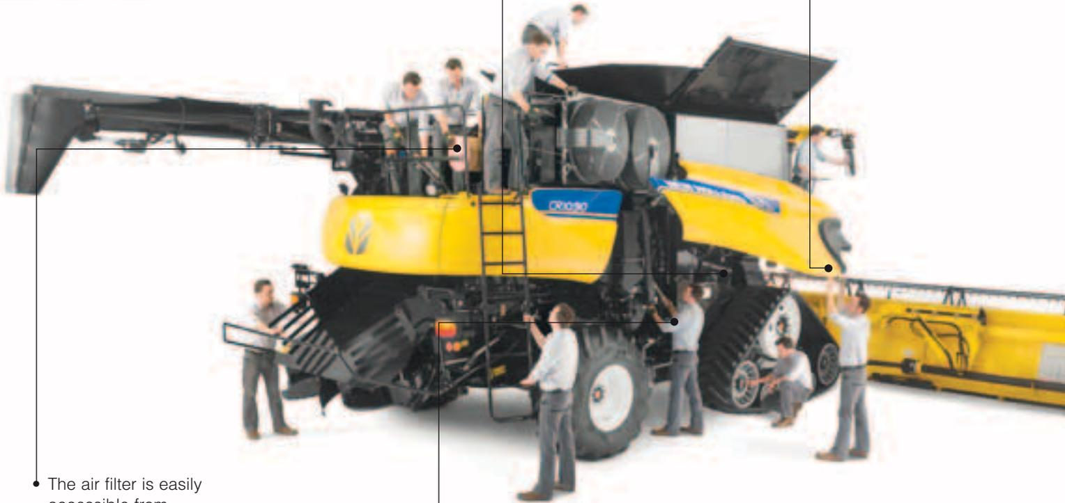
The air filter is easily accessible from the engine platform.
