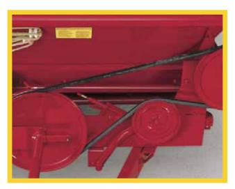
All models have a reliable straight-line V-belt drive that runs quietly and smoothly, eliminating the need for a slip clutch.
