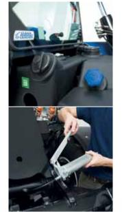
Access to the 140 litre fuel tank is via a wide opening filler, allowing in-field refuelling with cans if ever necessary. With a capacity of 27 litres, the AdBlue tank is large enough to last for at least 5 fuel tank fills.
