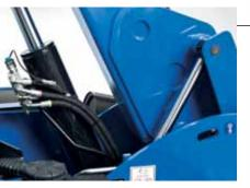
The boom hydraulic compensation cylinder is positioned to the rear of the boom and near the hinge point. The main lift ram is conventionally positioned under the boom. As the boom is raised both rams extend, but facing in opposite directions. This 'opposite working' helps to improve boom control, with additional benefits that include greater stability. The smooth action of the boom raise and lower reduces stress loads to enhance durability.
