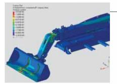
Based around twin U-shaped 10mm to 12mm thick sections, the completely new boom is immensely strong, with heavy duty pivot pins for optimum durability. New wear pads adjust quickly using a simple screw and lock nut design, without the need for special tools.
