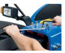
The once time consuming job of adjusting the telescopic boom pads has also been simplified, a simple nut screw and lock nut system making adjustment quick and easy.
