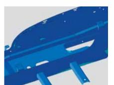
The one-piece H shape ladder chassis is made from 25mm thick, high tensile steel that is fully robot welded to ensure exceptional torsional rigidity. The boom support is exceptionally strong, its mass helping to counterbalance heavy loads.
