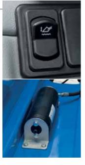
Boom suspension can be specified. The system is activated by the operator and is designed to help reduce shock loads when working over difficult terrain. The system automatically deactivates when the boom exceeds a 35 degree lift angle.
