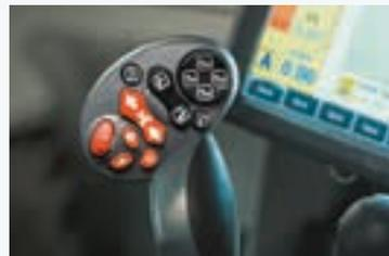
The soft-touch buttons feature backlight technology to make selecting controls in the dark even easier.
