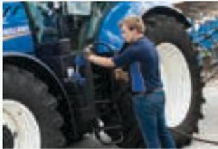
The 48 litre AdBlue tank's filler neck is narrower than that of the standard fuel tank, which prevents inadvertent filling with fuel. It only needs to be filled once every two refills of the fuel tank.
