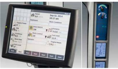
**INTELLIVIEW - GEAR AND SPEED AT A GLANCE** The standard IntelliView<sup>™</sup> display offers easy toggling between menus to display information that includes the exact engine speed and the selected transmission ratio. This information is duplicated by the 'A' pillar display, ensuring the operator always has key operating data to hand.
