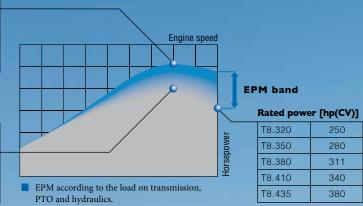
Rated powers are a useful reference but are usually surpassed by the max power figures during work, with or without EPM active.
