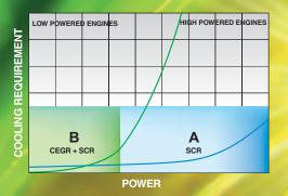
CEGR requires a cooling package to cool the hot exhaust gas prior to it being recirculated. Higher powered, larger capacity engines produce higher volumes of hot gas, which result in the need for a very large cooling package.
