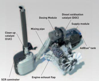
The key additional components of FPT Industrial's ECOBlue™ HI-eSCR system are:
