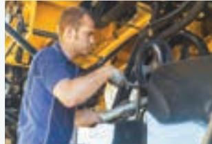
Easy ground-access to all oil filters and drain points and centralised greasing banks.
