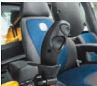
Shift button and ground speed unlock (behind).
