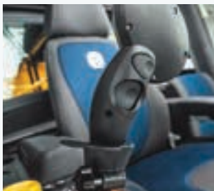
Shift button and ground speed unlock (behind)
