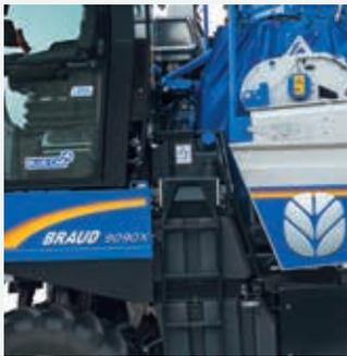
Two piece engine hood opens wide for full service access: front hood flips up perfectly for accessing the engine, side door swings with a gas strut for cleaning and servicing hydraulics and coolers.
