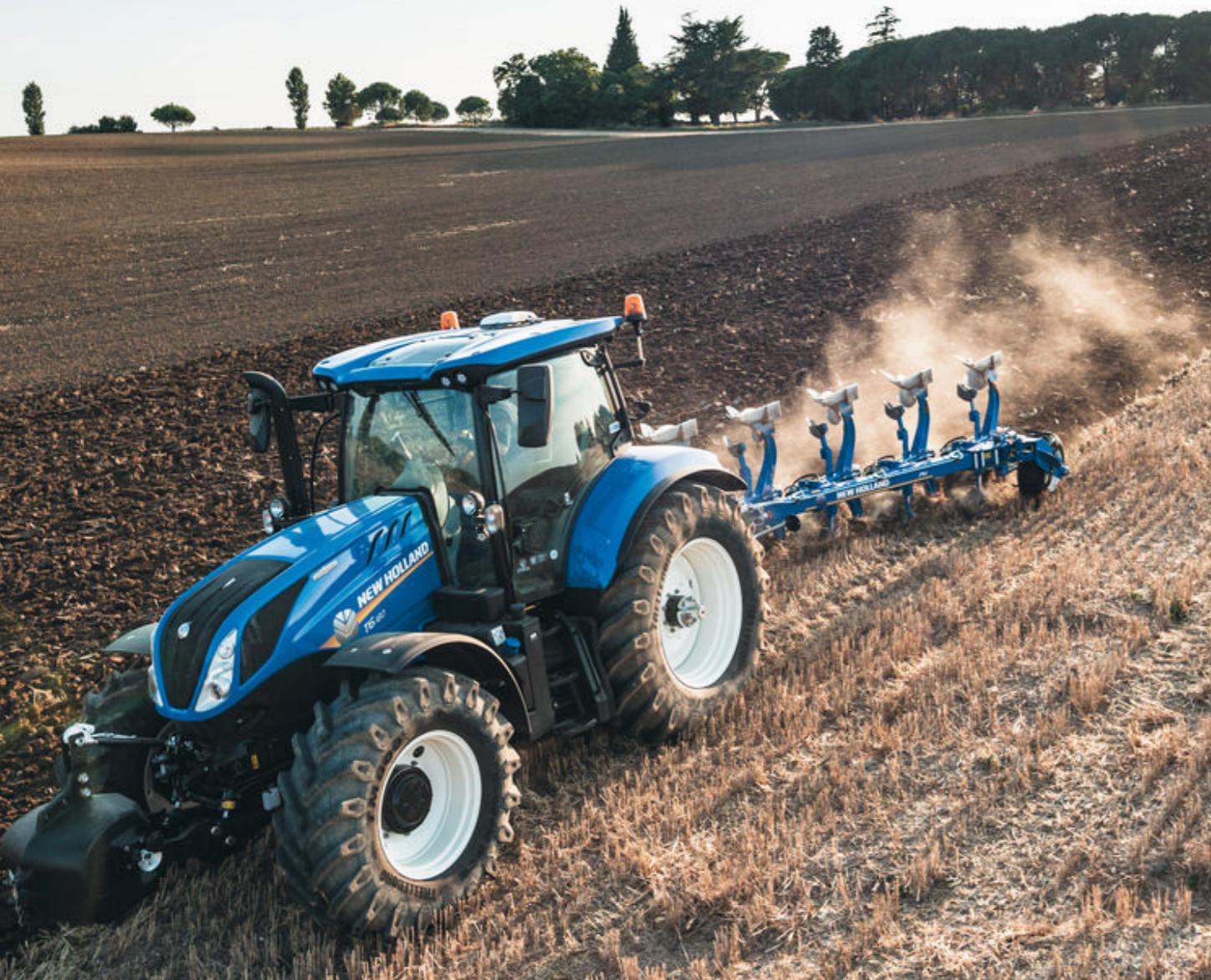
TrackXcontrol are unique plough and implement controls that enable to guide steerable implements precisely with RTK accuracy. Developed for CNHi guidance systems, the controls are compatible with almost all vario-ploughs, planters and equipment for mechanikal weeding and tillage. Precise guidance of the implements also relieves the driver, saves fuel and protects the plants in the row.
