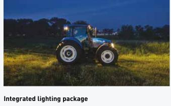
A full range of fully integrated work lights can be angled to suit any application. Shedding a broad spread of light, perfect for evening cultivation, the rear work lights are integrated into the redesigned roof for even easier access to low sheds and when working in areas of overhanging foliage. The intuitive controls are located on the B pillar.
