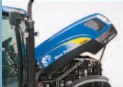
A one-piece, flip-up hood opens smoothly on a gas strut with open access to the engine, radiator, A/C condenser and filters.
