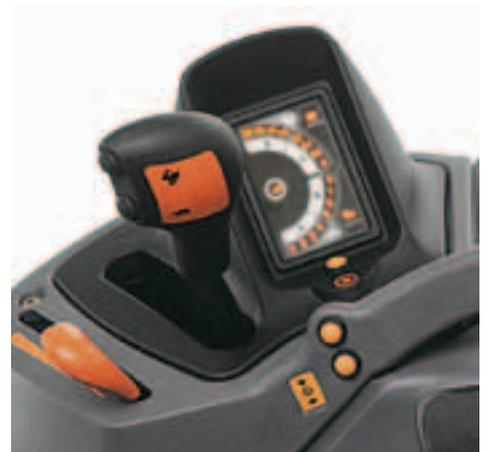
hydraulic powershuttle also lets you shift from forward to reverse without clutching for easier loader or grading work. Program the reverse gear you prefer for the work you're doing.
