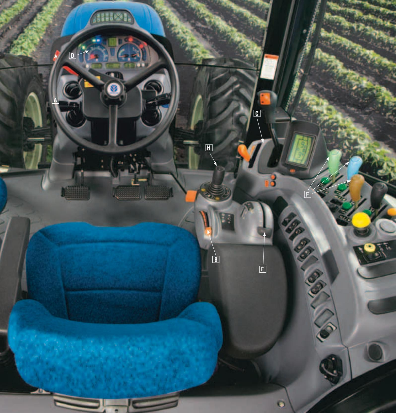
**D - Analog and digital instrumentation** and a series of 21 indicators and warning lights keep you informed at a glance.
