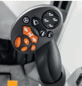
The soft-touch buttons feature backlight technology to make selecting controls in the dark even easier.
