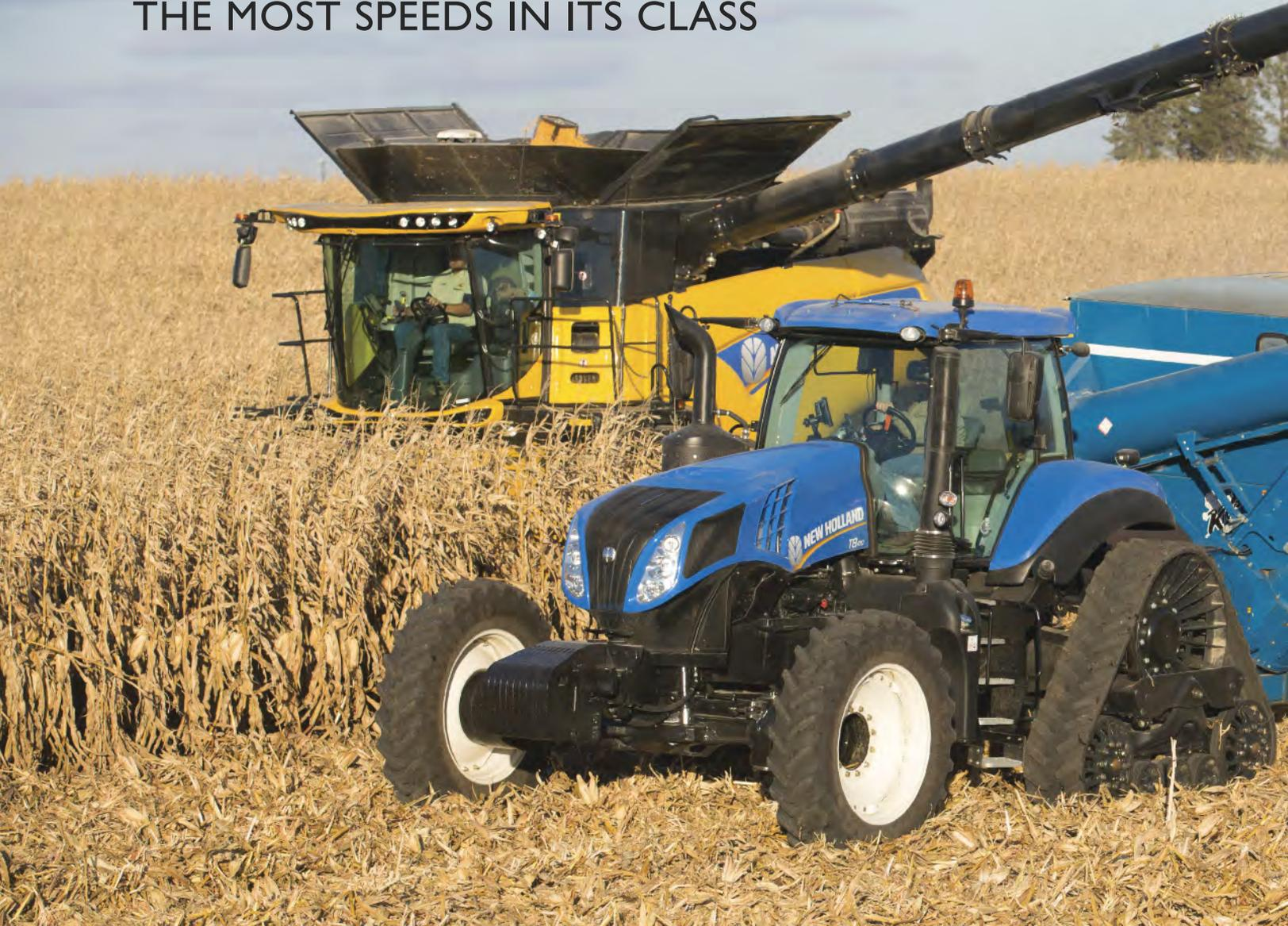
No matter which Ultra Command™ powershift transmission you choose, you get a minimum of 18 forward speeds, with eight of them in the critical 3- to 8-mph tillage range—more than other tractors in this class.
