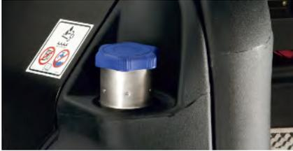
The AdBlue®/DEF tank capacity has been increased to 26 gallons and the diesel tank capacity has been increased to 179 gallons (163-gallon on CVT models) for more in-field time. The diesel tank is lockable for added security.
