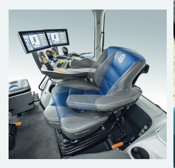
The **Dynamic Comfort™** seat boasts an enhanced low-frequency suspension mechanism. Stitched cushions, finished in a stylish cloth, feature two-stage heating for comfort in cold temperatures.
