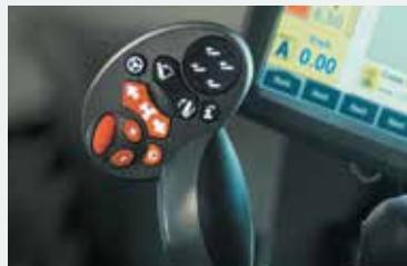
The soft-touch buttons feature backlight technology to make selecting controls in the dark even easier.
