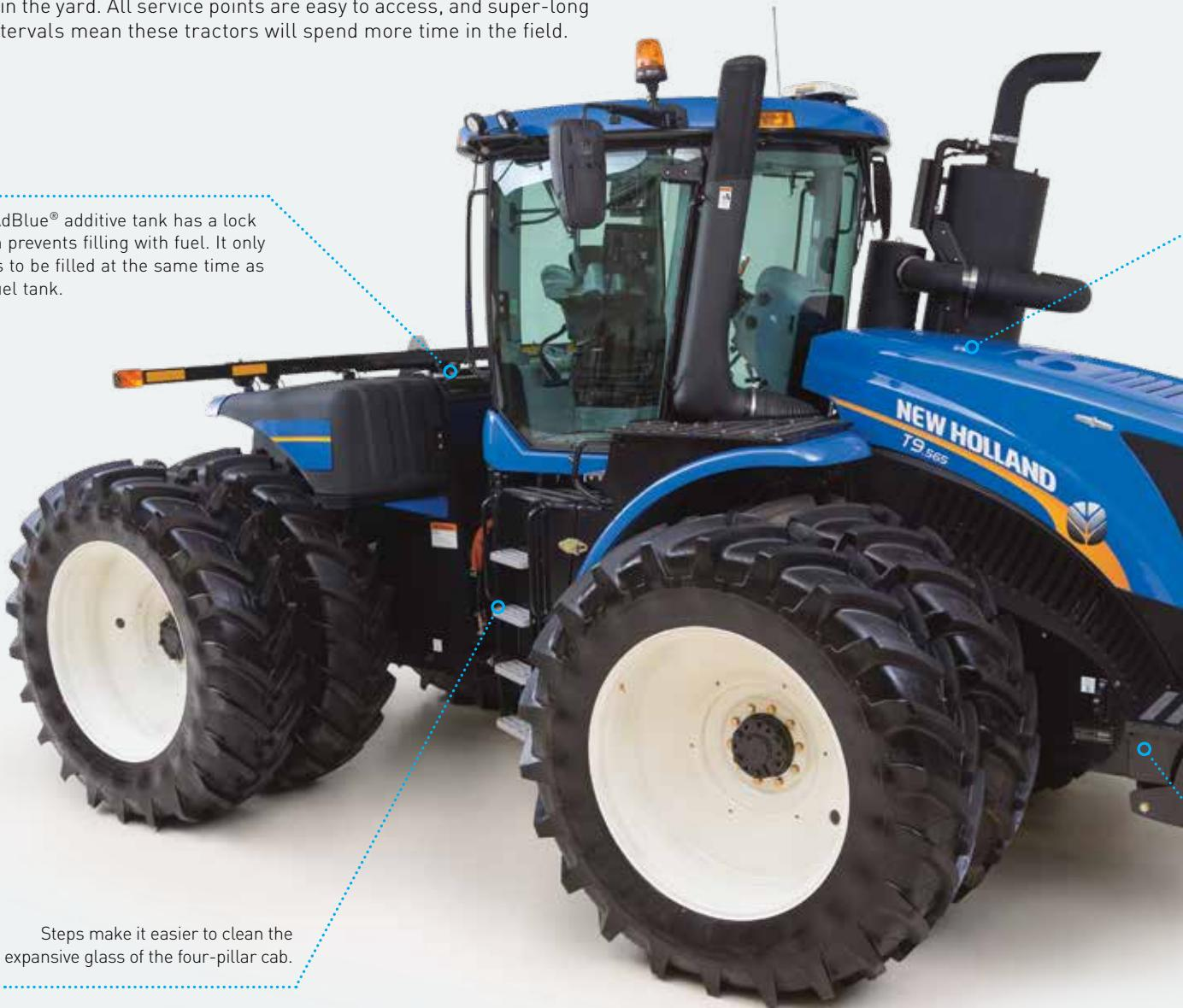
Steps make it easier to clean the expansive glass of the four-pillar cab.
