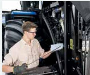
Engine and hydraulic oil check and fill points are easy to reach, making routine checks fast and servicing simpler. Engine service intervals have been extended by 100% to 600 hours.
