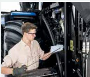
Engine and hydraulic oil check and fill points are easy to reach, making routine checks fast and servicing simpler. Engine service intervals have been extended by 100% to 600 hours.
