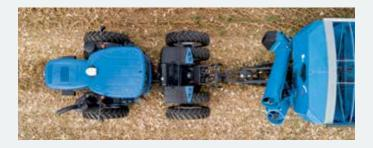
Grain cart applications with VF and IF dual tires (Row Crop Frame shown) allow for high-speed, low-pressure inflation, which lessens soil compaction while boosting fuel economy. Through less compaction, the T9 Series tractor improves your harvest and yields the following year.
