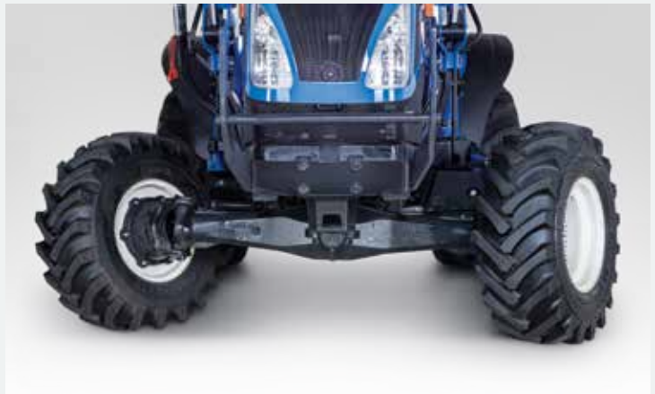
Engage the standard 4WD front axle electronically.
