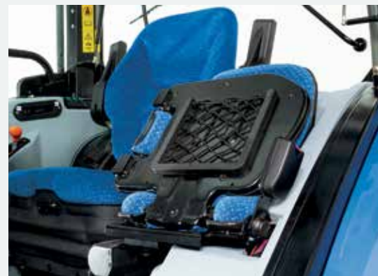
Comfortable air-suspension seat with armrests and fold-down instructor seat are standard.
