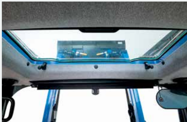
Dealer-installed High Visibility panel increases visibility to the loader.
