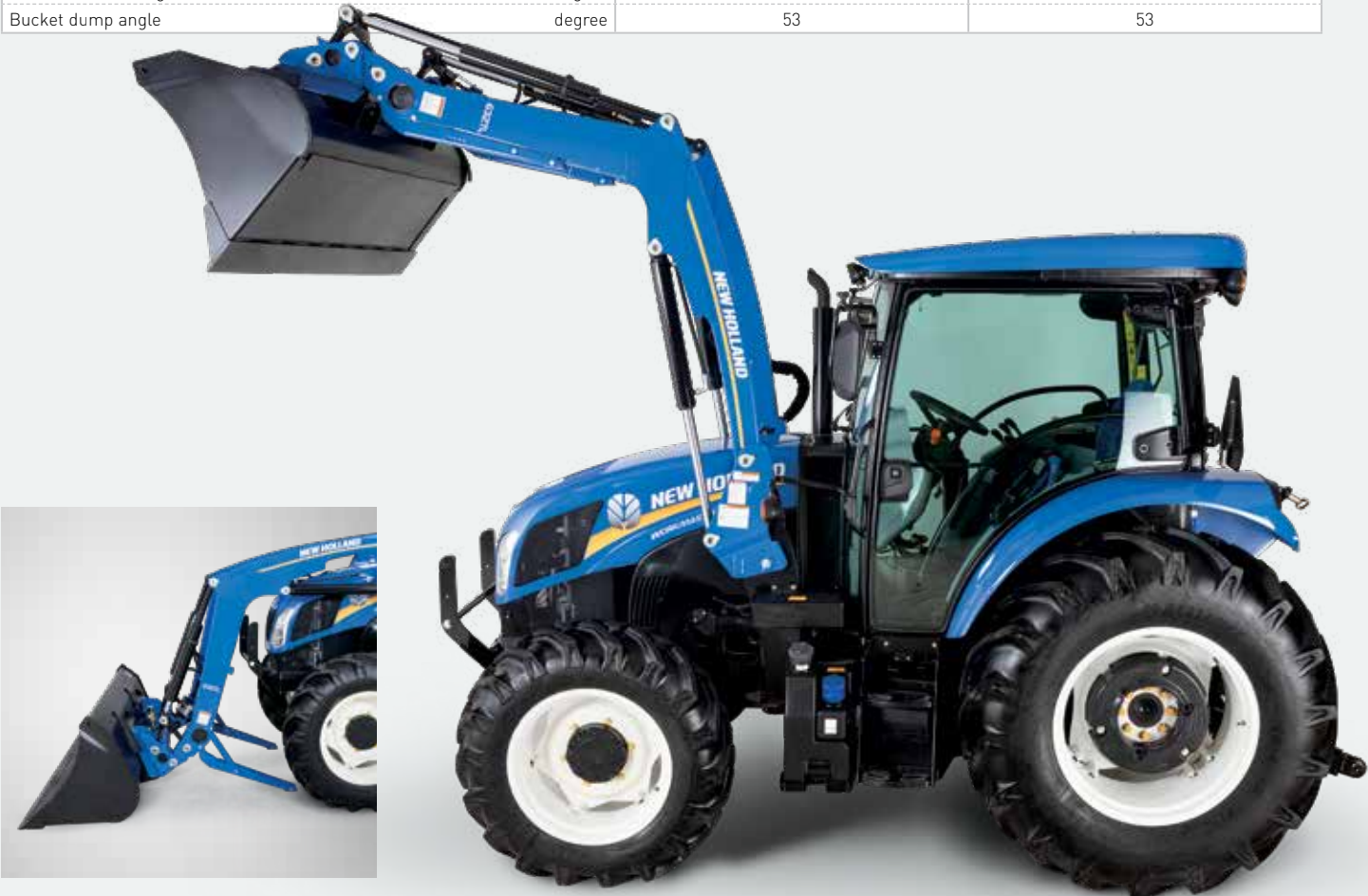
Parking stands deploy easily to allow quick removal of the loader.
