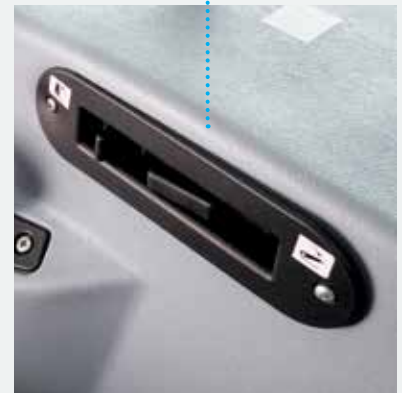
Lift-O-Matic™ 3-point quick raise control.
