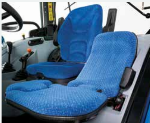
Comfortable air-suspension seat with armrests and fold-down instructor seat are standard.
