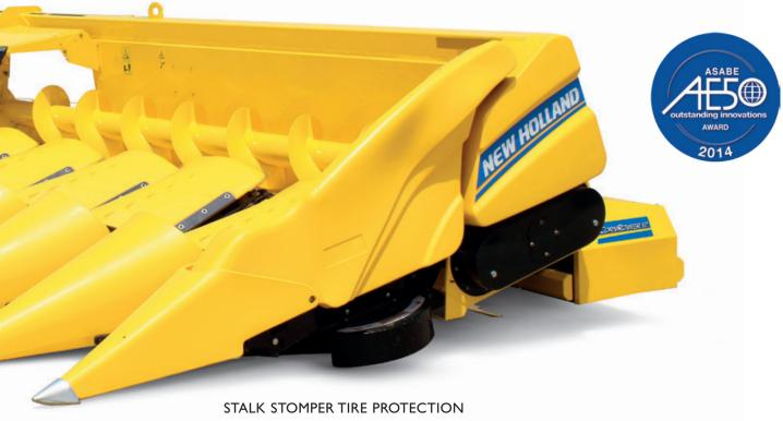
An optional Stalk Stomper kit is now available for fixed or folding corn headers to reduce tire or track wear when harvesting corn. Mounted on the header frame, the Stalk Stompers flatten the stubble in front of the wheels, greatly reducing the likelihood of punctures or uneven tire or track wear.
