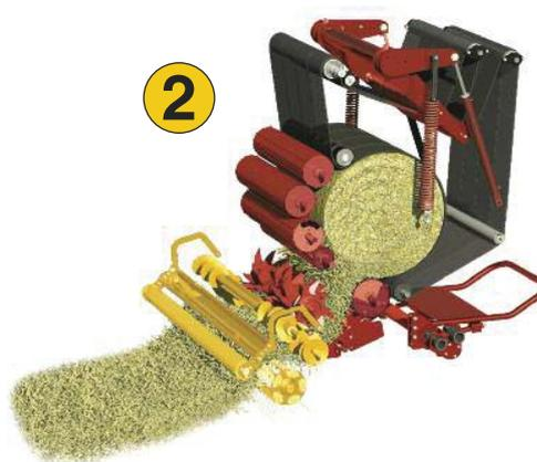
As the bale grows, the top rolls (G & H) pivot forward. The belt tension arm (I) also rotates to allow the bale chamber to expand. The belt tension cylinder (J) and belt tension spring (K) deliver reduced belt tension at the start to ensure positive core formation, even when baling short, dry crop.
