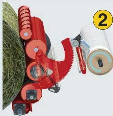
The duckbill pivots into the bale chamber between the fixed roll and pivot roll.
