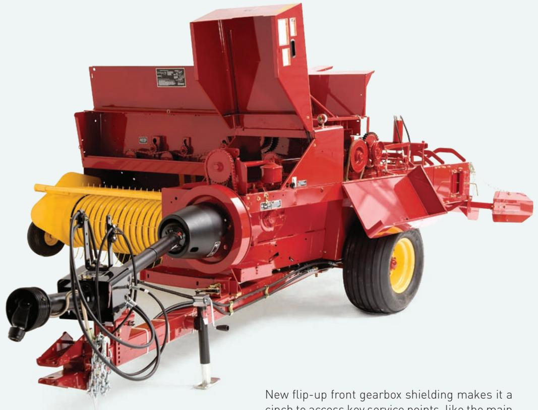
New flip-up front gearbox shielding makes it a cinch to access key service points, like the main gearbox and hydraformatic system.
