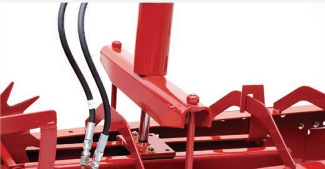
You can also equip your baler with hydraformatic bale tension control. This feature helps maintain uniform bale density in varying crop conditions.
