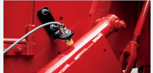
The automatic CropSaver applicator with stroke counter utilizes position sensors to detect when each bale is tied, the number of strokes per bale and determines the tons per hour harvested. Displayed on the monitor, this information allows the operator to adjust baling speed to maximize productivity and maintain an accurate bale length.
