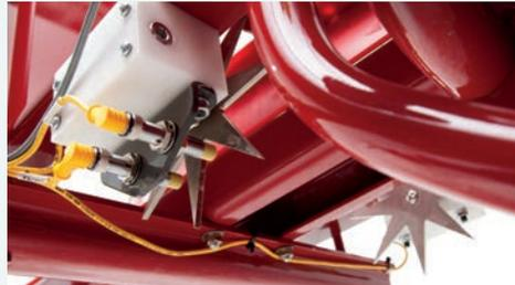
The automatic CropSaver applicators feature twin star wheels mounted on the underside of the bale chute that measure the moisture in each bale and continuously adapt the application rate every three seconds to respond to moisture changes.
