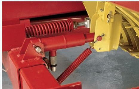
Hydraulic pickup lift. (Shown from rear of baler.) When baling, raise or lower your pickup as needed to adjust to differing terrain without leaving your tractor seat.
