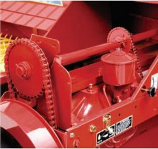
Hydraformatic oil pump is conveniently located for easier serviceability. (Models BC5060 and BC5070.)
