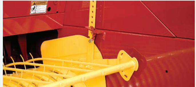
Pickups are manually raised and latched into transport position. Hydraulic pickup lift simplifies raising and lowering the pickup. It's standard on the BC5070 Hayliner and optional on other models.
