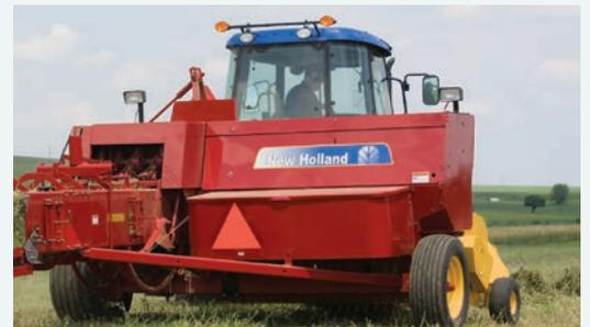
Road lights provide visibility when towing and turn signals for safety.
