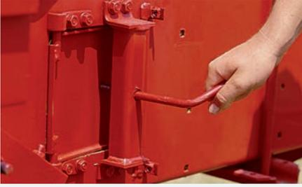
Adjustable bale tension doors on the BC5060 and BC5070 make it easy to change bale density at the bale case.
