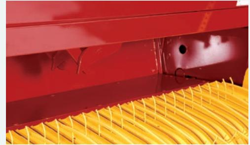
The replaceable feeder floor on all models provides wear resistance, easier serviceability, and extended baler life.
