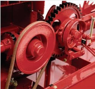
Redesigned knottor gear drive makes servicing or replacing the pickup belt simple.
