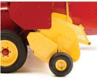
New pickup drive chain access shield provides easy entry for servicing. (Model BC5070)
