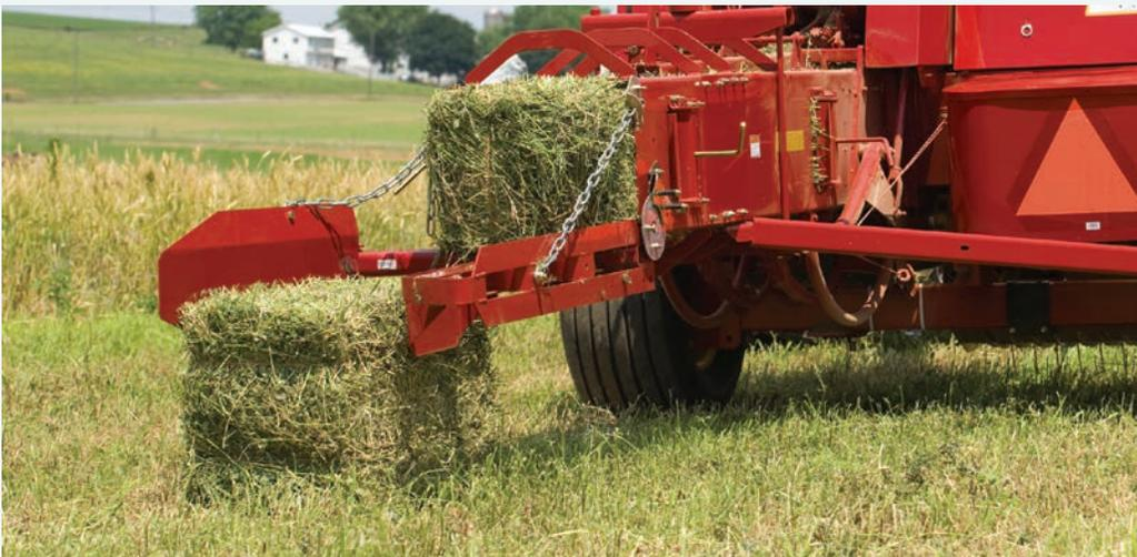
Quarter-turn bale chute drops bales on their sides so twine is kept away from the ground to prevent rotting. Sets bale into proper position for retrieval by automatic bale wagon. Bale case extension is also recommended when using the quarter-turn bale chute.
