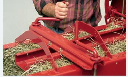
Tension springs are the economical way to adjust bale tension. A one-half-inch increase in spring tension equals 600 pounds of increased force.
