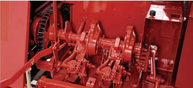
"Thousands of bales without a miss." It holds true for the dependable knotters and twisters that go on New Holland balers. Knotters and twisters are gear-driven for a simpler, easy-to-maintain design. Twisters are available on Models BC5060 and BC5070 only.
