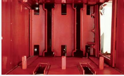
The rugged bale chamber is designed for better bale formation. Six hay dogs hold charges in place for firm, quality bales.
