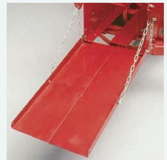
Triple-purpose chute supports bales as they leave the chamber; can be set to roll bales to the left, away from the next windrow. (Also becomes the base for bale-loading chute.)
