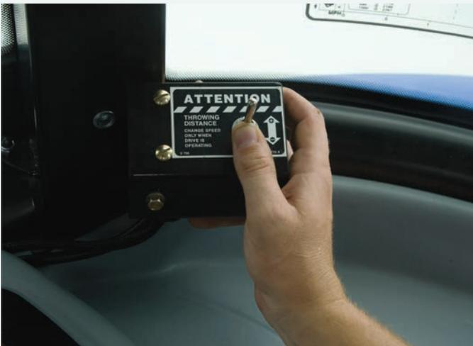
Distance and direction controller attaches to the tractor. The toggle switch controls the speed of the throwing belts for distance.
