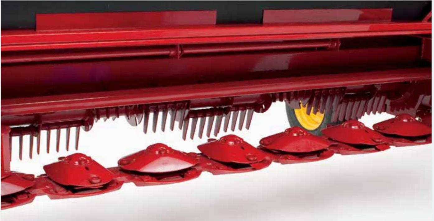
H7000 side-pull Discbine® disc mower-conditioners mow cleanly and smoothly through tough conditions. Featuring the classic and reliable MowMax cutterbar, these Discbines have cutting widths of 9' 2" and 10' 4". Like the newer MowMax™ II cutterbar, the classic MowMax cutterbar features the New Holland true modular design with ShockPRO™ disc drive hubs.
